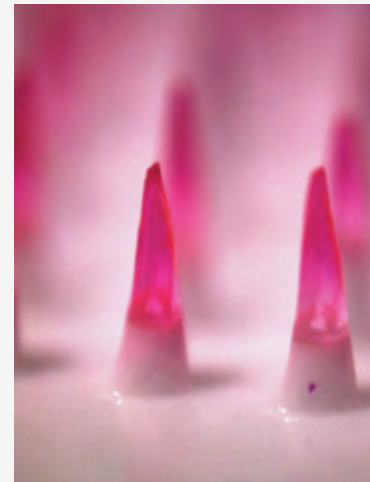
LEFT: A patch containing 36 dissolving microneedles is shown on a fingertip. Courtesy of Georgia Institute of Technology/Jeong-Woo Lee; RIGHT: Microscope image shows dissolving microneedles encapsulating a pink dye. The microneedles dissolve within minutes after insertion into skin to release encapsulated drug or vaccine. Courtesy of Georgia Institute of Technology/Sean Sullivan
