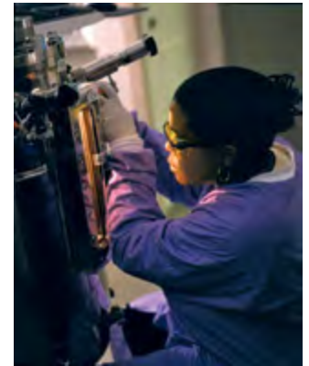
Biologist checks culture volume in a fermenter growing Pichia pastoris yeast. This culture medium expresses a malaria antigen that the lab is evaluating for possible vaccine development. Courtesy of NIAID
